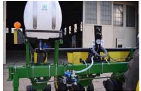
Finished rig: Tank, ground drive pump, manifold, pressure gauge, and hoses
